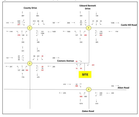
Figure 3.5: Scenario 1 total traffic with proposed development – PM Peak Hour
